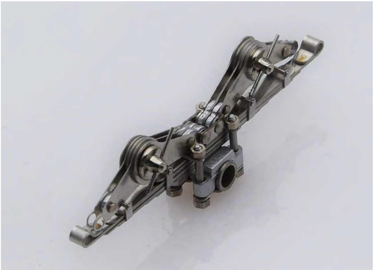
As in the original, the leaf spring consists of a thick spring assembly; the friction dampers made of several layers of metal.
