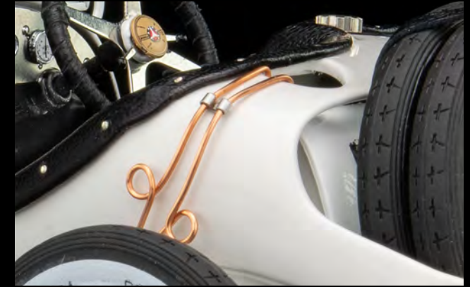
External gasoline pipes.
