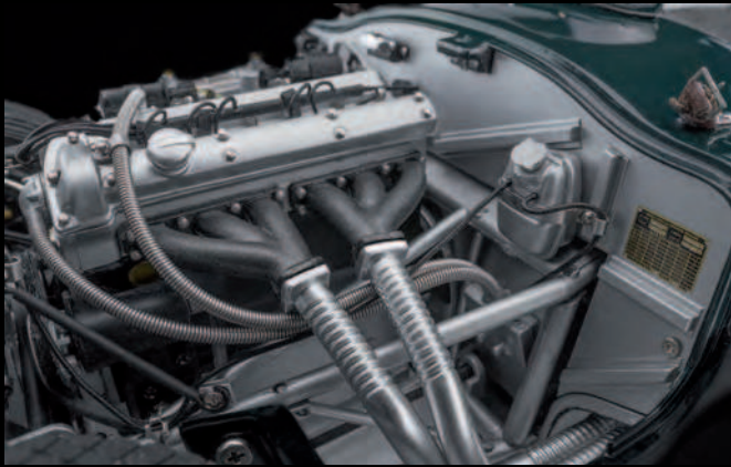
True-to-the-original replication of the six-cylinder in-line engine with all accessories and wiring. Metal exhaust pipes.
