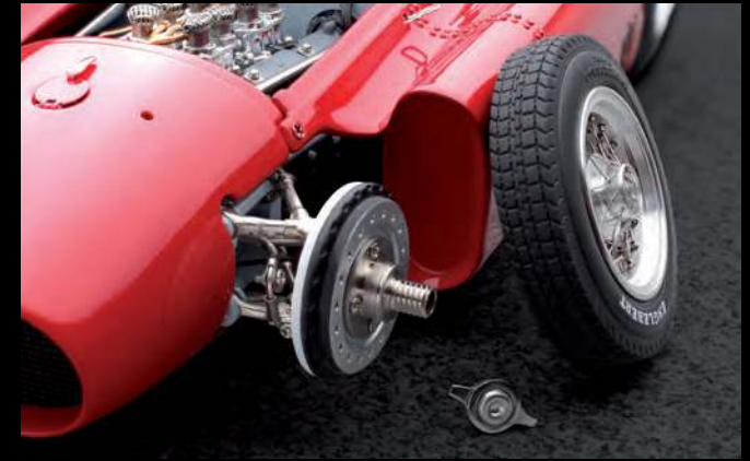
Modern wishbone front suspension with finely ribbed brake drum. The wheels can be removed from the model.
