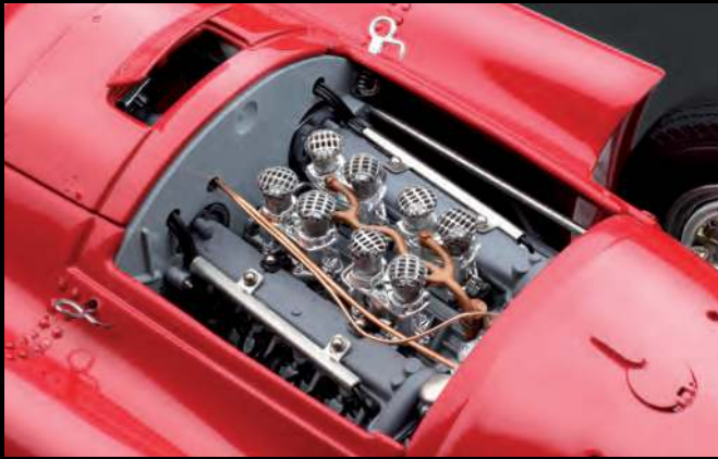
The engine was designed as a supporting element and was offset 12° around the longitudinal axis to the left to allow the cardan shaft rotating at crankshaft speed to move past the pilot and across the De-Dion axis built-in gearbox. Characteristic was the transaxle principle, four overhead camshafts in a lightweight and compact 90°-V8.
