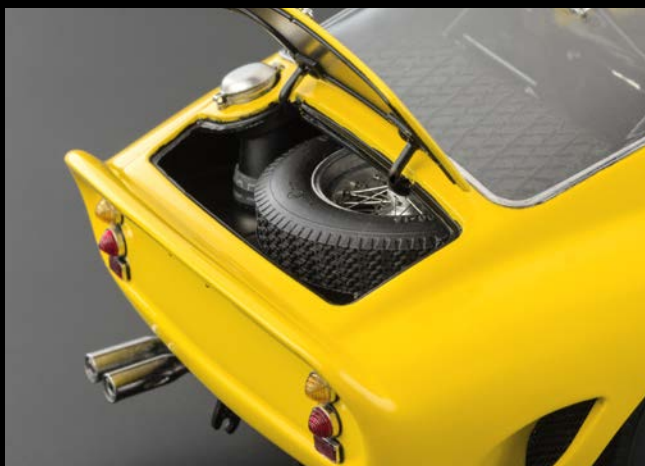
The removable spare wheel is located well secured in a receptacle.
