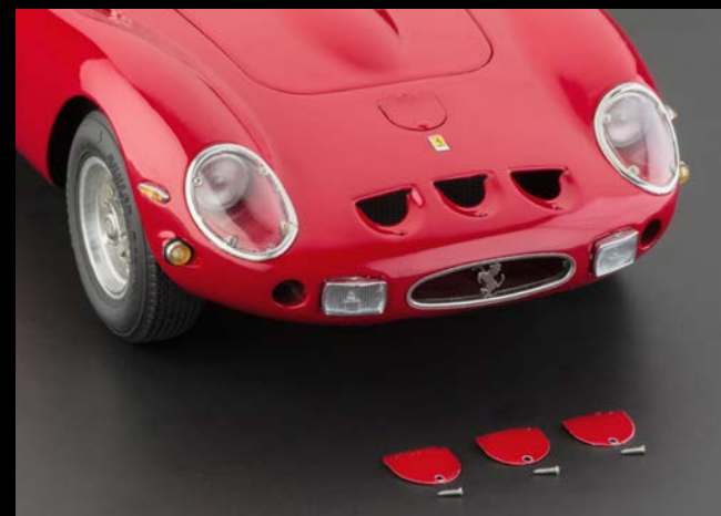
3 lockable covers for the additional air intakes above the radiator grille, also removable if needed.
