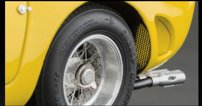
Rear fender with ventilation opening for heat dissipation of the brakes. Prototypical light alloy wheel.
