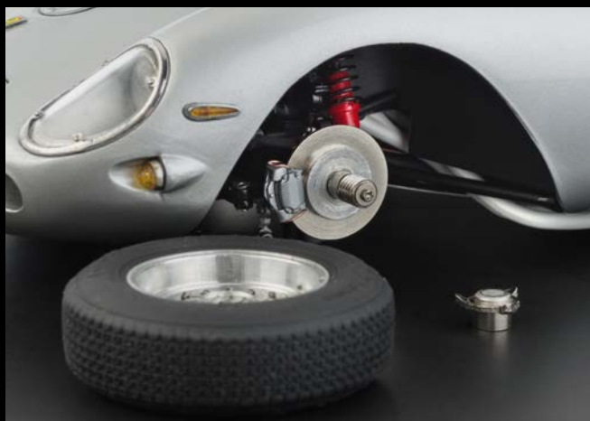
The wheels are removable (3-wing central-locking-nut) and open the view on the disc brakes.
