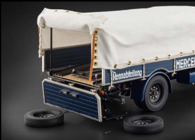
Openable side boards and tailgate and detachable tarpaulin, fastened with fine leather straps.
