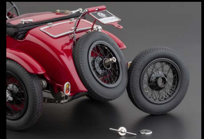
Functional brackets for holding the two spare wheels. Loosening a tommy screw releases the spare wheels.
