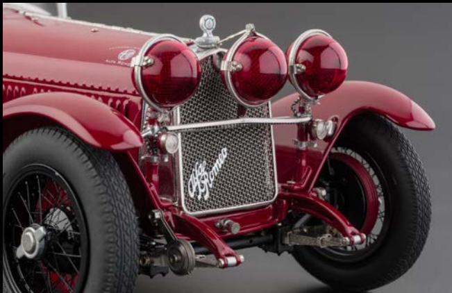
Distinctive Alfa Romeo front end with the famous triple-headlight unit. Headlights fitted with mesh guards against stone-chip damages. The red caps are removable.
