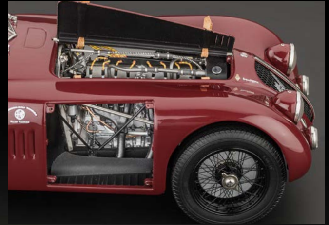
Highly detailed 8-cylinder in-line-engine with crankcase made of two light-metal blocks, each with 4 cylinders.
