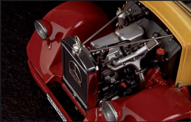
Beautifully rendered four-cylinder Diesel engine with all attachments and complete cable laying.
