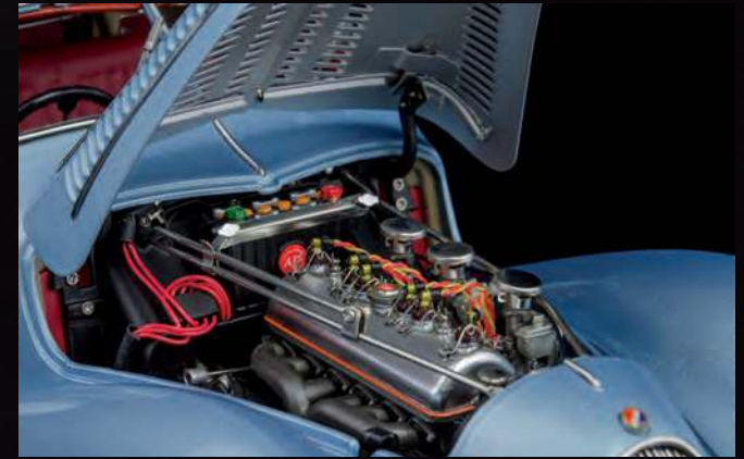
A work of art beneath the bonnet as well: A six-cylinder in-line engine with carburetors and all the attachment units and lines.
