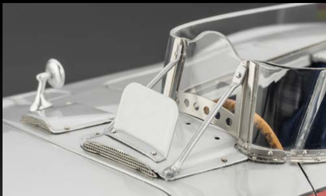
Fangio and Kling drove without a co-pilot. Their cars were equipped with a metal cover over the co-pilot's seat. Kling's car had an additional stone guard in front of the wind shield.
