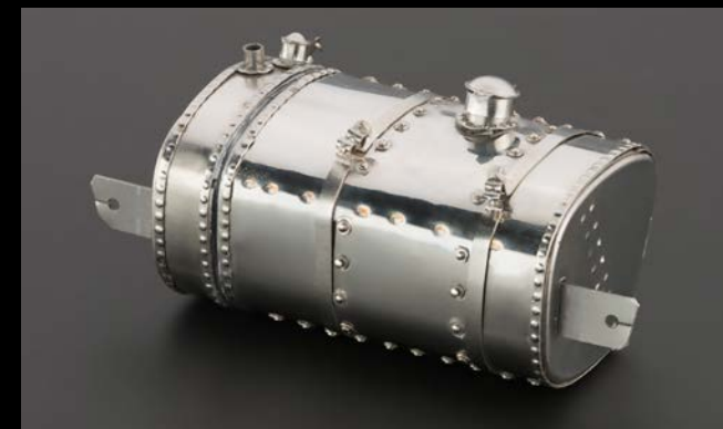
Gas and oil tank are made of stainless steel plate and hand-assembled with an elaborate rivet arrangement.
