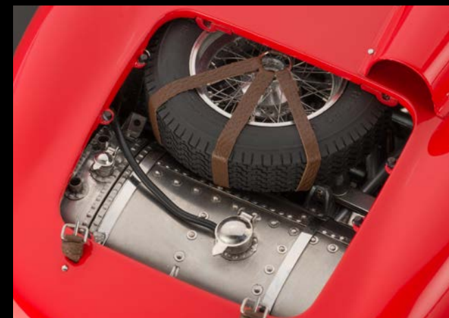
The spare wheel is fastened with three leather straps, as in the original vehicle.
